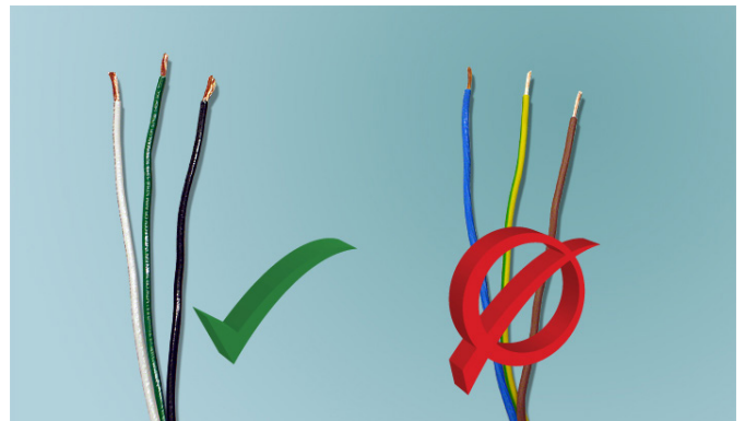
Cable/circuit wire, North American standard
