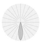
Fixture luminous flux:6658lmFixture luminous efficacy:116lm/WOptical distribution:symmetrical
