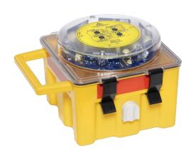
Obelux Low-Intensity Portable (LI-P) is a portable, battery-operated red obstacle light. Optionally, it can emit infra-red light in addition to red light. Obelux LI-P has been designed for outdoor use and has enclosure made of shock-proof polycarbonate.
