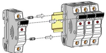
Gang multiple poles to meet application requirements using kit catalog number  $\mathsf{JV-L}$  (gangs up to four poles).
