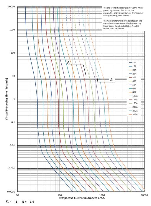
170M - Sizes 000 to 3, DIN 43620, Dual indicator fuse links, 690 V a.c. (IEC), 700 V a.c. (UL), 10 A to 1600 A
