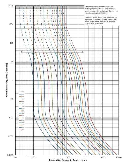
170M - Sizes 000 to 3, DIN 43620, Dual indicator fuse links, 690 V a.c. (IEC), 700 V a.c. (UL), 10 A to 1600 A
